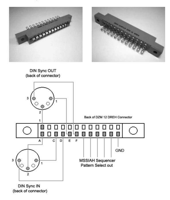
The user port connector is a 12/24 pin edge board connector with .156" (3.96 mm) spacing. These are available from a number of manufacturers such as Sullins, Compar etc. Use a 5 pin male DIN connector for the sync IN. Though depicted as a male connector you might want to use a female one for sync OUT. In that case, remember that pin 1 and 3 are mirrored. Sync OUT is optional, you do not need it to slave the MSSIAH to your Sync24 equipment.
