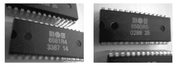
The 6581s have a printing on the top saying 6581. R3 or R4 means Revision 3 or Revision 4. On the left picture above, the SID in question is a 6581 Revision 4 (good!). The right picture shows an 8580 which is always revision 5.
