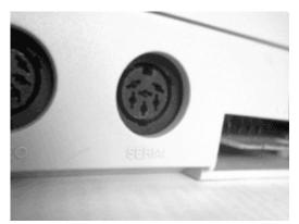
**Serial port** ("IEC") This is where to connect the disk drive. Some printers use this port too.
