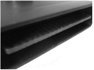
The word "Terminals" refers to the part of the circuit board sticking out of the bottom of the cartridge.
