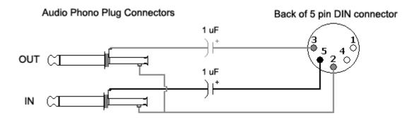
The 1 uF capacitors are from the SID specs. Their purpose is to improve the sound quality. With a fairly high S/N ratio and ground noise level, the caps do not really make any noticeable difference to the SID's audio output.
