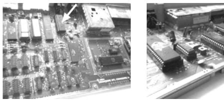
6581s are located to the left of the "RF modulator" (TV output) as seen in the left picture whereas 8580s are located just below it (right picture).
