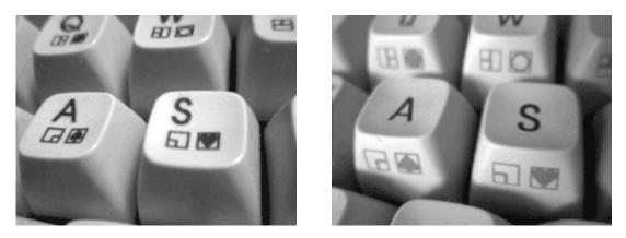
You can spot a late C64 by the symbol letters printed on the top side of the keys (left image) as opposed to old commies where symbol letters were printed on the vertical side (right image). Don't trust this method too much though. Keyboards as well as audio circuits in the computer might have been switched. It's merely a first notice of what might be a nice purchase when looking at an ad for a used C64.
