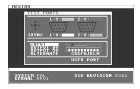
The upper part of the *Diagnostics / Ports* screen shows the Controller ports (joystick, potentiometers and mouse) and the lower part is a user port tester. Use **CRSR** keys to select port status and press **RETURN** key to execute.
