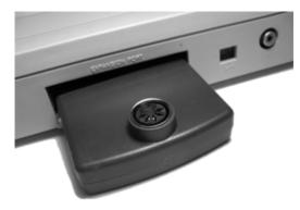
3: Gently push the cartridge all the way into the expansion port
